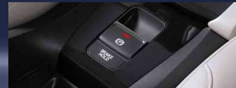
Electric Parking Brake with Auto Brake Hold
