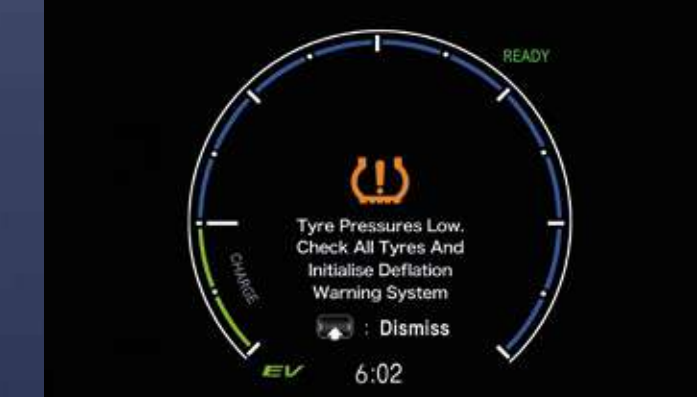
Tyre Pressure Monitoring System (Deflation Warning System)
